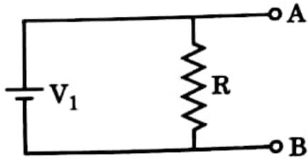
The current through the resistance R is very close to 1 mA and the voltage across point A and B,  $V_{AB} = 1$  V. Now the circuit is changed to:
