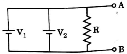
where value of  $V_2 = 5 V$ . The internal resistances of both the batteries are  $0.1 \Omega$ . The current through the resistance R is about:
